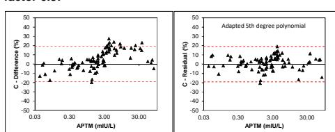
%-Difference and %-residual plot for assay C with unmodified data
